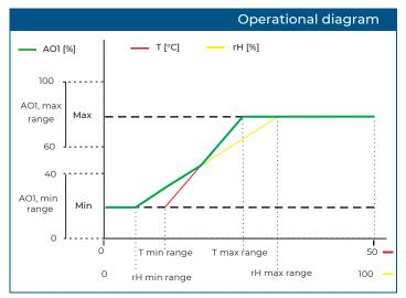
Note: The output changes automatically depending on the highest of the T or rH values, i.e. the highest of the two output values controls the output. See the green line in the operational diagram above. One or multiple sensors can be deactivated. E.g. it is also possible to control the output based on the measured temperature only.
